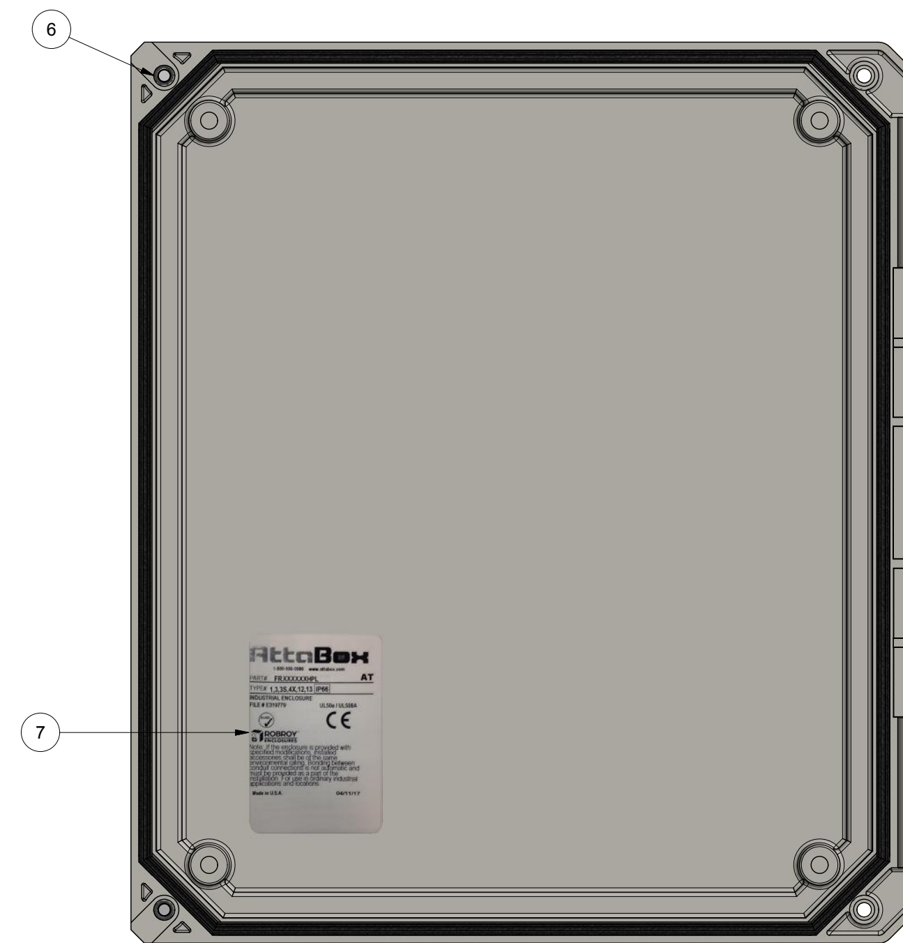
BACK SIDE (1) MOUNTING FOOT REMOVED FOR CLARITY TORQUE SCREWS TO 25 IN.-LBS
