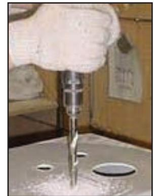
Using a drill with a positive rake angle and thin points or split points can help reduce cutting pressure. Feed rates must also be constant and may even be reduced upon exiting from a hole to reduce flexing of the part when the drill exits. Using a solid back surface to support the part when drilling can also aid in reducing delamination and chipping. Caution on polycarbonate to not generate enough heat that the material starts to melt or string.
