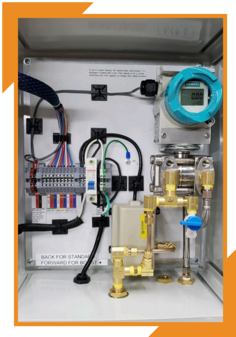
Interior of Automatic Bubbler System made with AttaBox Industrial Enclosure
