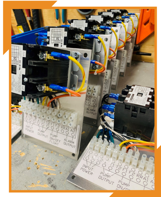
Pump controls meant to be housed inside AttaBox Industrial Enclosures
